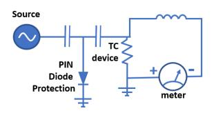
temperature, which are then converted into changes in voltage. As signals become large (around 20dBm) un-checked device temperatures would exceed a few hundred degrees centigrade and impact device lifetime. A protection diode was added to mitigate risk and enable use of the full dynamic range; shunting away high-power RF signals Which help to maintain device temperature (protecting the silicon and metal films).
