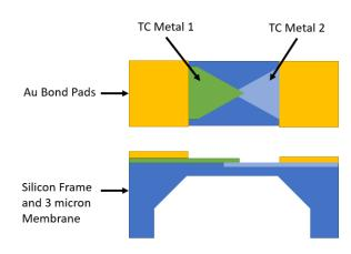
The thermocouple device is manufactured with standard MEMS processes followed by flip-chip bonding to a low loss substrate.
