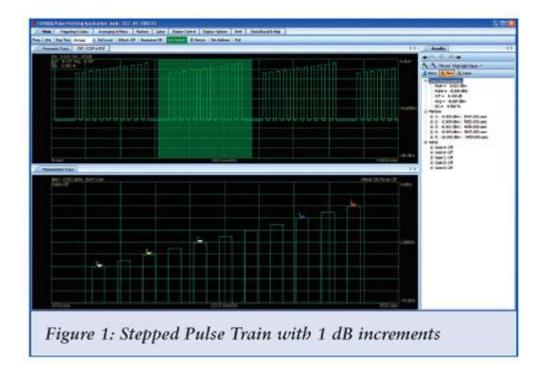
Power sensors must include pulsed measurement capabilities and achieve performance specifications to meet the requirements needed for these applications. LadyBug Technologies provides this capability and performance in a compact USB power sensor: its LB480A Pulse Profiling USB PowerSensor+TM includes dedicated software with all the tools necessary for complete power characterization of pulsed and bursting signals.
