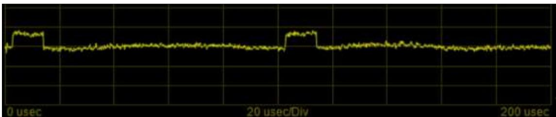
*Figure 6 Low Level Pulsed Signal with 100 Averages Applied*
