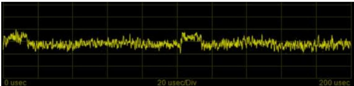
*Figure 5 Low Level Pulsed Signal with 20 Averages Applied*
