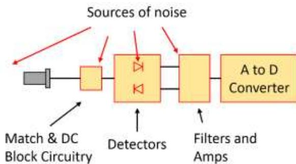
*Figure 2 Power Sensor Front End*
