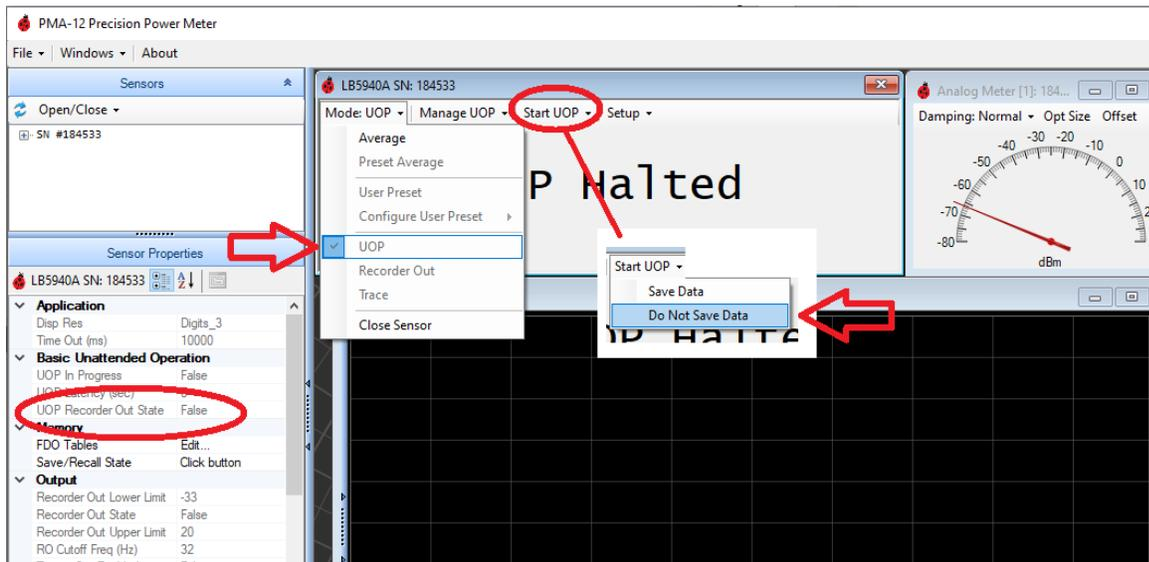
**Figure 2 - Recorder Out in Unattended Operation**
