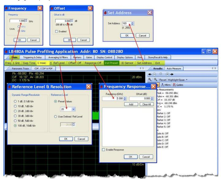
**NOTE**: The reference level and resolution settings change the formatting of the data that is presented whereas offset and response modifies the measured values.
