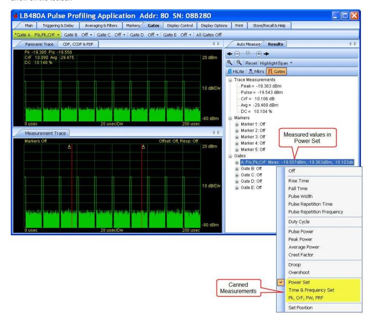
**NOTE**: You can always highlight the span if you drag the cursor over the Panorama view (or select a highlight span percentage and start time) even if you are in markers or gates mode. To highlight in the Measurement view you must be in the highlight mode. If you do not switch to highlight mode before clicking/dragging in the Measurement view you may inadvertently reposition markers or gates.
