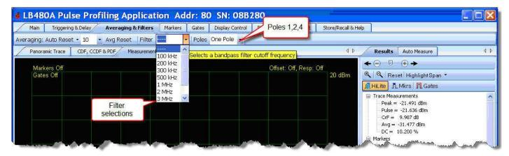
The number of **Poles** has the effect of determining the sharpness of the frequency roll off depending on the filter selection. The greater the number of **Poles** the steeper the roll off and again, the reduction in the high frequency component of the signal. More **Poles** then decrease roll off but have the affect of increasing both the rise and fall times of the displayed signal (as time relates inversely to frequency).
