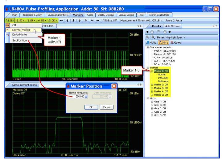
Only one marker can be active at a time although all five markers (or marker pairs) can be displayed simultaneously. The active marker will have an asterisk (\*) next to its number in the toolbar and the marker number will be underlined and appear slightly larger in the display.
