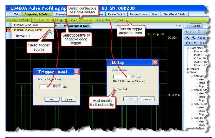
**NOTE:** An incoming pulse must be on at least 0.20 usec followed by at least 1 usec of off time for the sensor to properly trigger.
