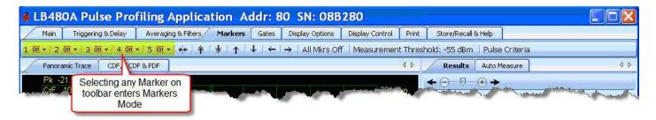
To manipulate (move or place) a particular marker the mouse pointer must be in the **Markers** mode. Because pointer modes are changed quite often there are a number of ways to change modes as shown above. You can select the **Markers** mode in four ways:
