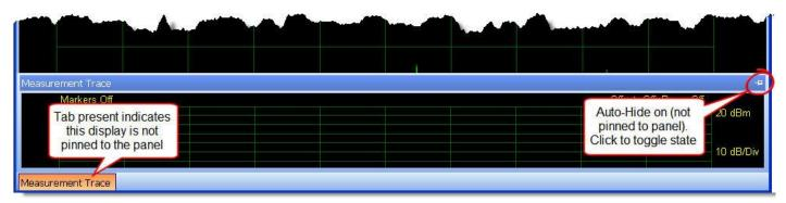
**NOTE:** A docking tab must be pinned or, in other words, Auto-Hide must be off in order to move it to another location.
