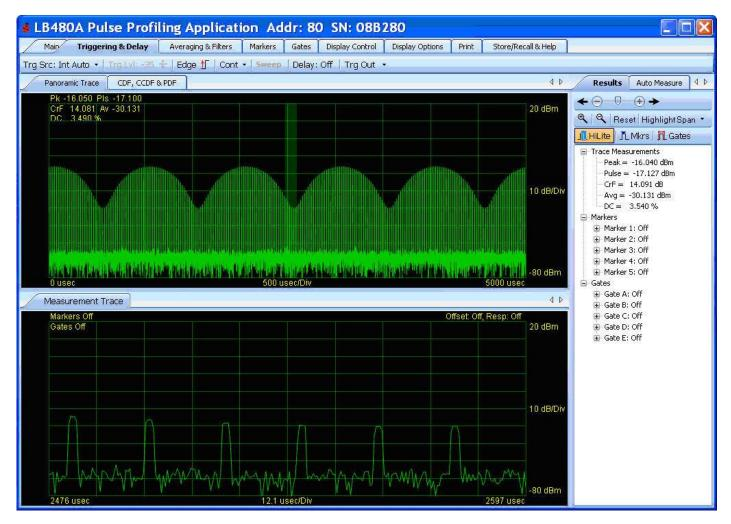
**NOTE:** An incoming pulse must be on at least 0.20 usec followed by at least 1 usec of off time for the sensor to properly trigger.
