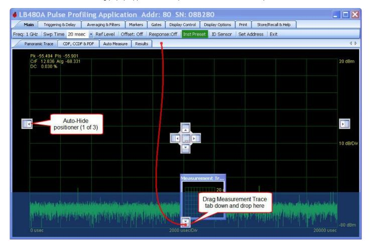
The **Measurement Trace** will move to the position indicated with Auto-Hide active as shown below. This means the display is not pinned to the panel and you must point to the Measurement Trace tab to view it. Toggle the Auto-Hide icon to turn this feature off or to pin the pane to the panel for continuous viewing.
