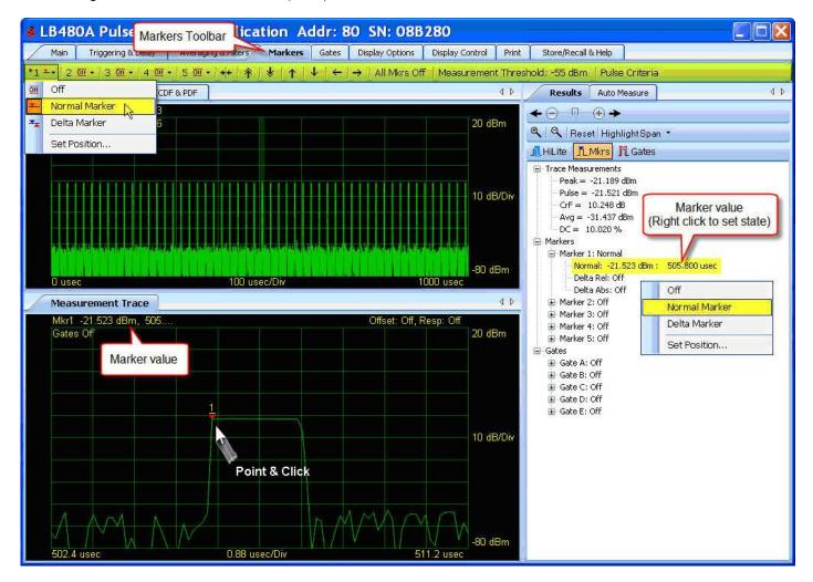
**NOTE**: Only one marker can be active at a time. The active marker will have an asterisk (\*) before its number in the Markers toolbar. The marker tree in the **Results** pane will not show the active marker.
