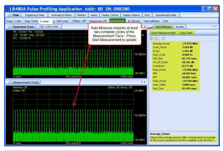
**NOTE:** The **Auto Measure** feature requires at least two complete cycles of the pulse to be viewable in the **Measurement Trace** window.
