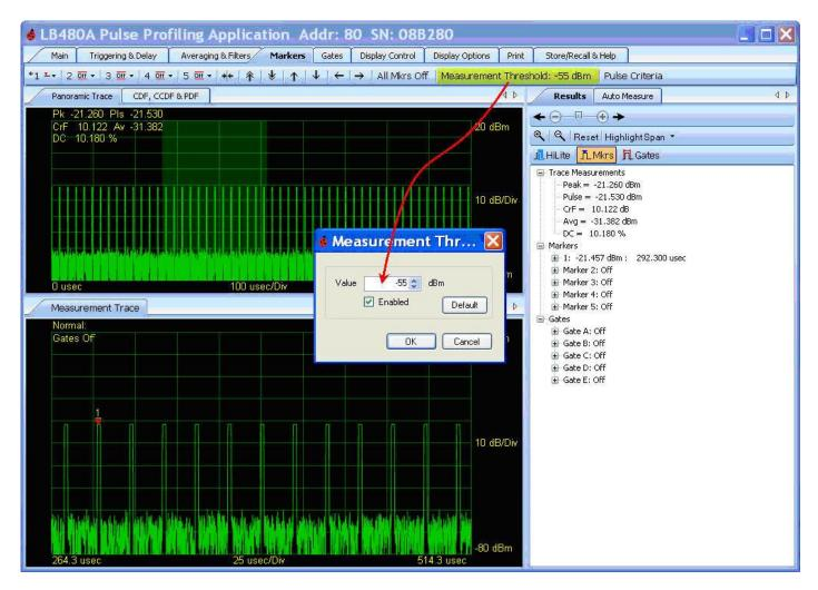
*EXAMPLE*: Set **Measurement Threshold** to -20 dBm. Setup a normal marker on top of the pulse. Click **Marker to next peak right** and notice the active normal marker requires the threshold value to be met before it will search for the next peak. Since our signal is below -20 dBm it will not move. Set the marker threshold back to the default value (-55 dBm).
