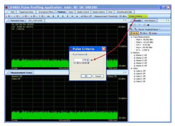
**NOTE:** The **Pulse Criteria** definition stated above applies to data used in both marker and time gated measurements.
