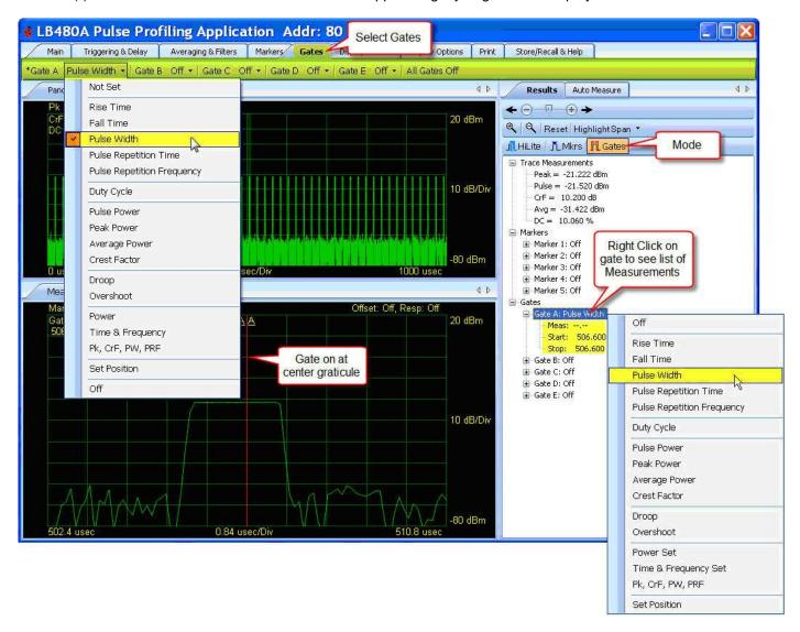
**NOTE**: You can always highlight the span if you drag the cursor over the Panorama view (or select a highlight span percentage and start time) even if you are in markers or gates mode. To highlight in the Measurement view you must be in the highlight mode. If you do not switch to highlight mode before clicking/dragging in the Measurement view you may inadvertently reposition markers or gates.
