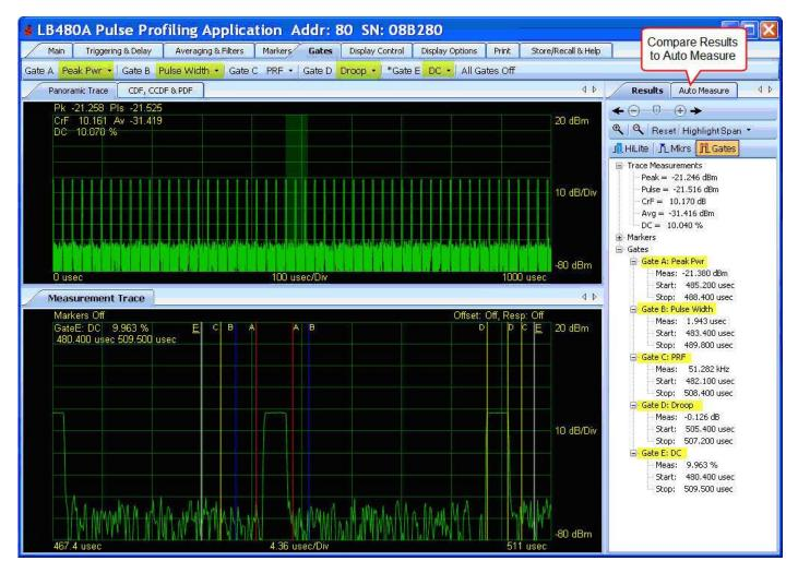
**NOTE**: You can always highlight the span if you drag the cursor over the Panorama view (or select a highlight span percentage and start time) even if you are in markers or gates mode. To highlight in the Measurement view you must be in the highlight mode. If you do not switch to highlight mode before clicking/dragging in the Measurement view you may inadvertently reposition markers or gates.
