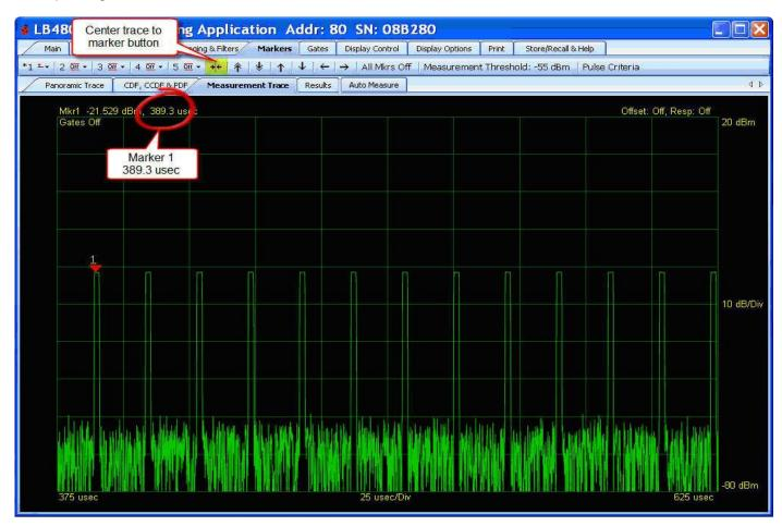
**NOTE:** The marker search will be affected by continuous waveforms whose pulse characteristics vary in amplitude so as to cause the search to jitter on instantaneous peaks. You can stablize the trace may switching to single trigger. Refer to the **Triggering & Delay** toolbar for setting the trigger source.
