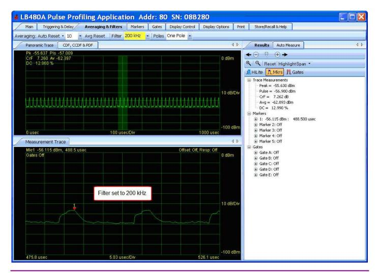
**NOTE:** The Filter and Poles selections are only active with LB480A Option 004. Otherwise the selections will be inactive and set to 100 kHz and one pole.
