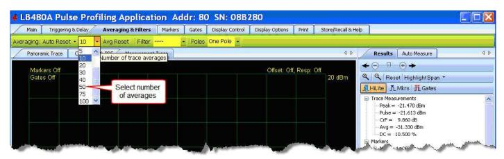
**Auto Reset** triggers an averaging restart when the trace changes are pronounced (it assumes a new signal is being examined). **Manual Reset** makes this function discretionary for the user. Shown below is an example of averaging OFF compared to averaging set to 10 and the effect. Increasing the number of averages increases the measurement time.
