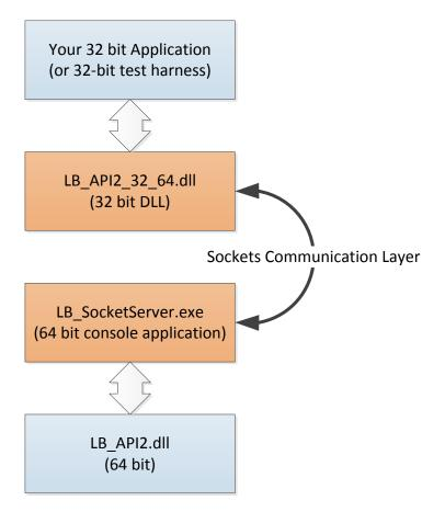
The solution we chose was to interpose a sockets communication layer between the 32 bit application and the 64 bit LadyBug API. The interface seen by the 32-bit application is, in general, identical to LB-API2.dll interface. Three calls have been added to the interface:
