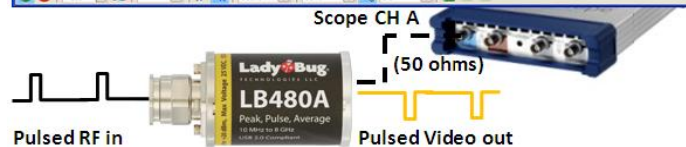
Measuring Opt 0W2 Wideband, Negative Detector, Analog Video Output Signal
