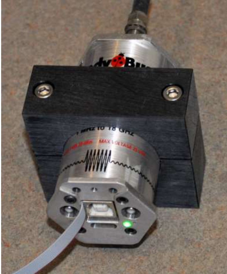
Figure 4. LB5918A with SPI Connection in Action.
