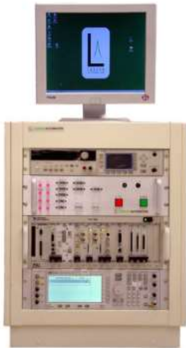
Figure 1. Modern 802.11 Communications Test Set. Courtesy Larson Automation.
