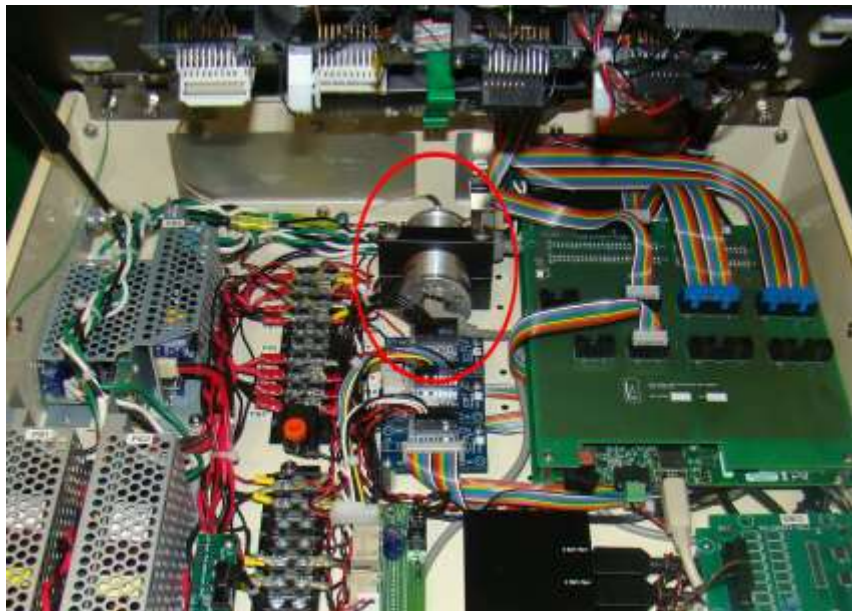
Figure 3. Test set for wearable devices. Courtesy Larson Automation.
